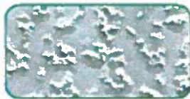
SEM photo, 8um Diamond Lapping Film (150X)
