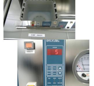
4.2.27 Remove the stainless lid from tank 2 (see below) and place basket in the solvent strip bath for 2 minutes.
