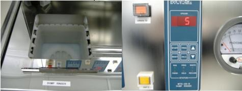
4.2.20 Remove the stainless lid from tank 2 (see below) and place basket in the solvent strip bath for 2 minutes.
