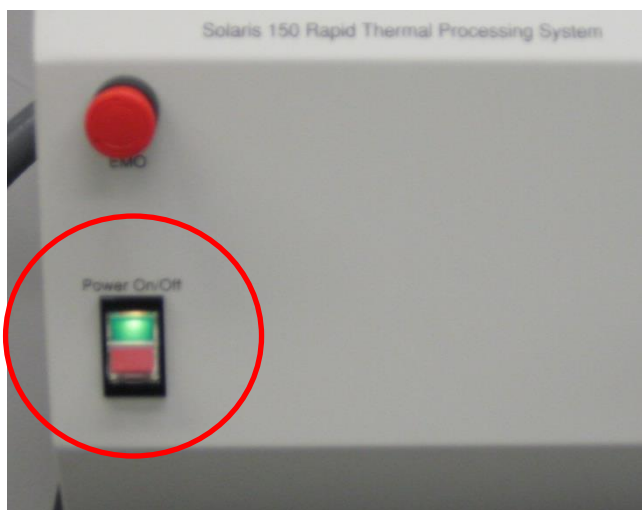
Figure 2. Main oven power switch and EMO button.
