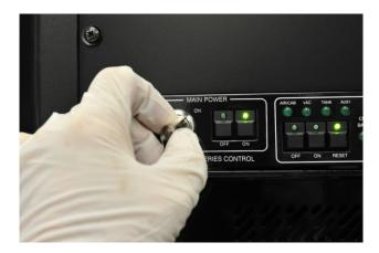
Step 3: In the "High Voltage" section press the "Reset" button.
