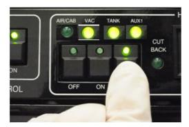
Step 4: Check that the VAC/Tank/Aux 1 lights are lit. The Air/Cab interlock light will light after approximately 5 minutes. Wait for this to happen. You can work on sample prep while waiting.
