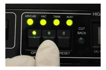
Step 6: Ensure the DC/Kilovolts readout shows voltage. \_\_\_\_ Do not change the voltage.
