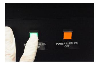
Step 2: Turn the "Main Power" key to on, then press the "On" button.
