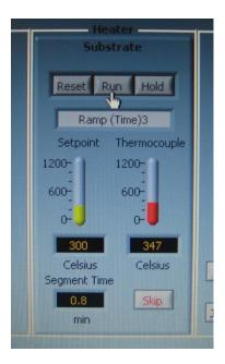
The substrate heater will go through a preprogrammed heater ramping routine to the requested temperature. Wait for the temperature to stabilize at set point before proceeding with the deposit (return to Step 3)
