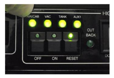
Step 5: Once the Air/Cab light is on, press the "On" button. Do not press lightly; press firmly with no hesitation.
