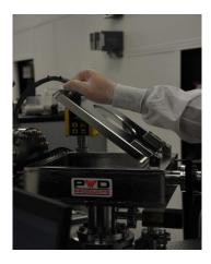
Step 4: Place the properly prepared (see sample prep section) sample holder on the loader arm; the posts on the loader arm (one on the right ant two on the left) should correspond with the slots on the sample carrier. Check to ensure there is there is no debris on the o-ring; if there is debris; clean the o-ring an isopropyl alcohol moistened wiper.
