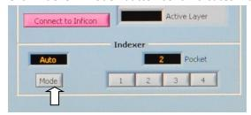
4. Click the "4" button and watch the motor on the left of the machine drive the hearth feed through to ensure it rotates completely.
