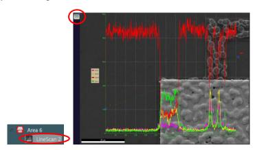
9.7. Clicking on a point in the line scan will bring up the spectrum for that point (which can be saved as already described); the selected point on the line scan will be indicated in the image. However, if you want to save the image with the superimposed line scans with the selected point indicated, this must be done via screen capture, rather than by using the folder icon.
