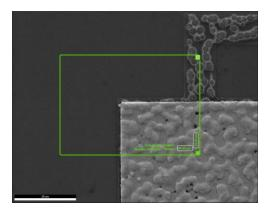
8.3. Hover over "Collect Map" and select desired options for "Resolution" and "Quality" ("256×200" and "Standard" are usually sufficient). Select "Collect Map" to start mapping; the system will auto identify the elements present in the region and then begin mapping.
