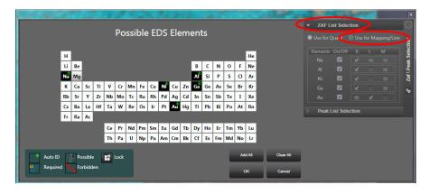
8.7. To change the color of a particular element being mapped (while mapping), select "Display Options" and then "Assign Element Colors". Then select the element of interest from the periodic table and assign the desired color to it. Keep in mind that this will be color assigned for this element for all other maps or line scans in the project (unless the assigned color is changed again).
