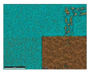
8.6. To add/remove elements for mapping, first make sure "E2P" is selected from the compass and then select "Modify element list" (above the compass). You can then add or remove elements using the interactive periodic table. Additionally, by expanding the "ZAF/Peak Selection" tab on the right side of the periodic table, you can also choose which peaks you want to use to map for each element ( $K_{\alpha}$  versus  $L_{\alpha}$ , etc.).
