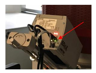
4.3. If it has been determined that the EDS detector is not properly communicating with the TEAM computer, open "Device Manager" and expand "Network Adapters"; then disable and enable "Intel Gigabit CT Desktop Adapter #2".
