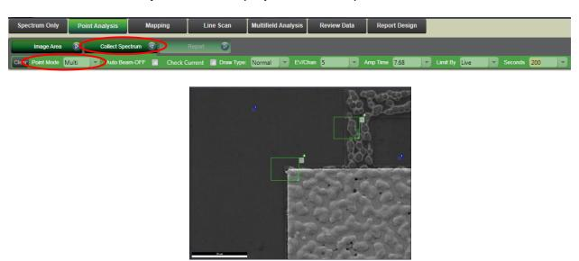
7.4. Double clicking on the area in the project tree used for point analysis will pull up the reference SEM image used for point analysis with all spots/regions used for analysis indicated. To save this image to your designated folder, hover over the image and select the folder button (top left side of the image); the spots/regions used for point analysis will be saved on the image.
