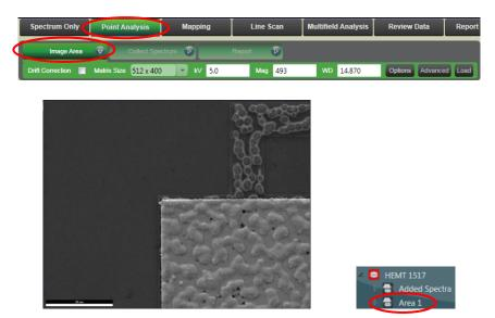
7.2. Hover over "Collect Spectrum" (the same settings used for "Spectrum Only" mode will automatically load); under "Point Mode", you can select options to analyze single or multiple points. If the "Single" option is selected, just click on the image (or click and drag to define a rectangular region) and analysis will start automatically (the spectrum will save to the project automatically once complete)
