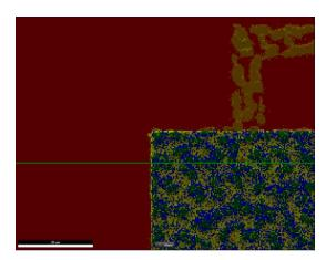
8.5. To change to a composite map of the individual elements, select "E2P" from the compass (lower left corner of the window).
