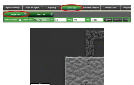
9.2. Hover over "Collect Line" and select a value for "Resolution" (distance between points on the line. The smaller the value of "Resolution", the greater the number of points on the line, and the longer the time required to complete the line scan. For "Quality", the "Standard" setting is usually sufficient.
