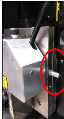
Figure 4 Hybrid Head release screw
