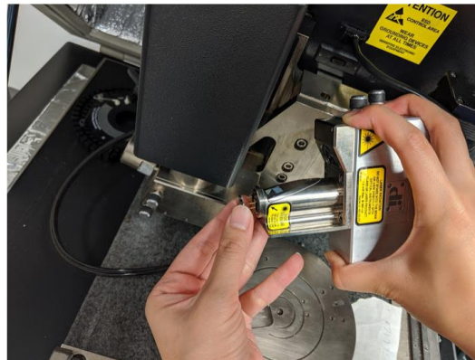
Figure 5 placing tip holder onto the head
