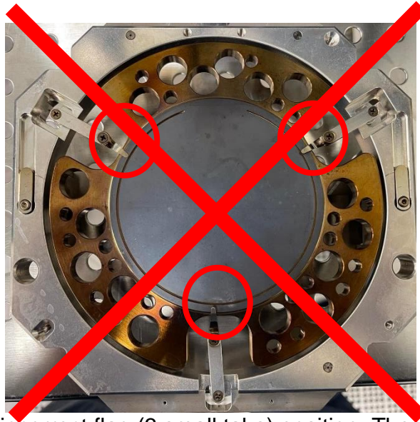
Figure 5. Example of incorrect flag (3 small tabs) position. These need to not be over any part of the inner ring.
